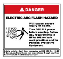
Figure 1 - Minimum Required Labeling
